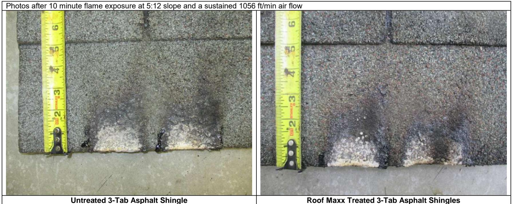
**Remarks:** Initial flame was more intense with the Roof Maxx treated specimen even though the resultant flame spread was not appreciably different from the untreated specimen. Post-testing, the plywood deck of the Roof Maxx treated sample sustained a flame, whereas the untreated flame extinguished quickly upon removing the gas torches.
